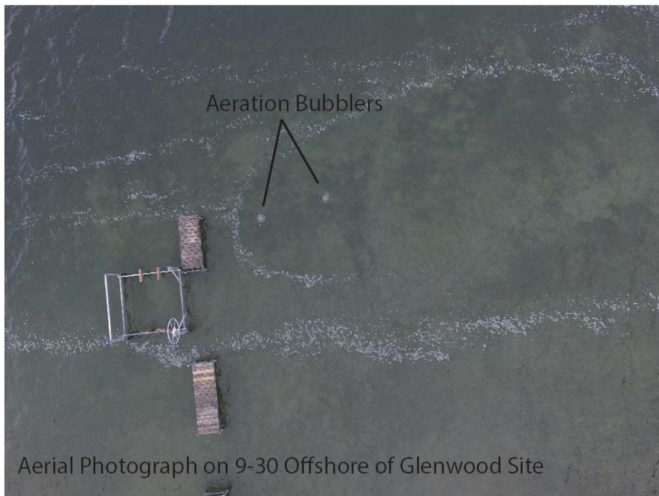
Fig. 12. BGA circles and white-foam streaks displaced around the aeration bubbles at the Yacht Club (above) and Glenwood (below) sites. It suggests that the aeration bubbler devices push surface accumulations of materials up to ~30 meters (~100 ft) away from the bubbles, even on windy days.
