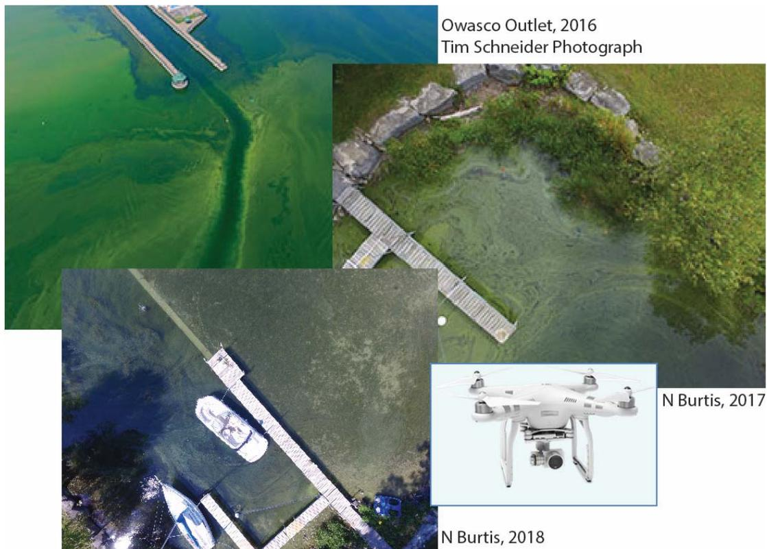
Fig. 6. Drone images of significant BGA blooms from previous years (above) and no bloom during 2018 (below), conclusions confirmed by water samples. The bottom and top right-hand images were from the identical site. The intensity of the green in the earlier images greatly exceeds the worse bloom imaged by drone in 2018.
